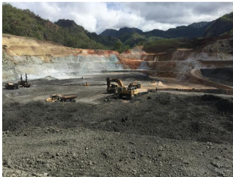
Image 1 – Excavating blasted material in Kali Kuning pit
