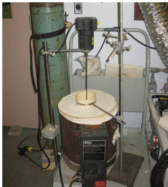
FIGURE: 2kg agitated roast test setup in Canada.
