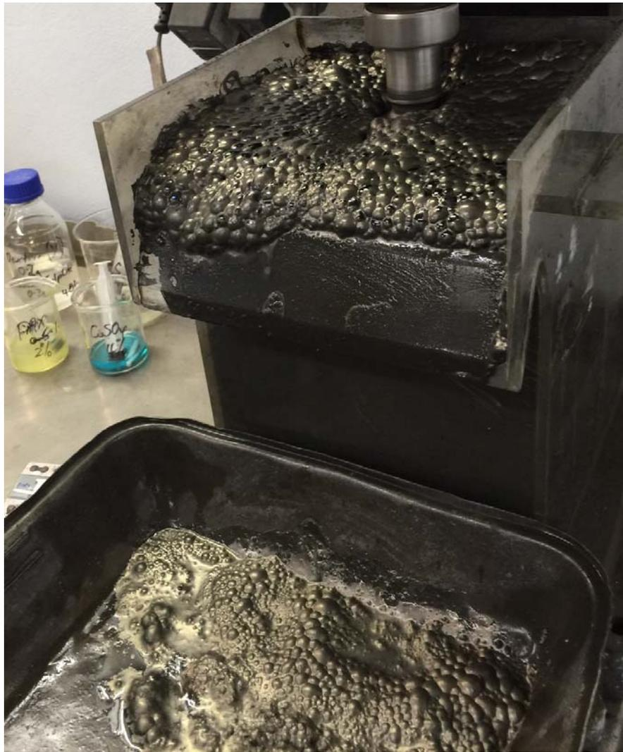
Figure 2. Sulphide Cleaner Float from Cleveland Tailings Bulk Sample at ALS Burnie
