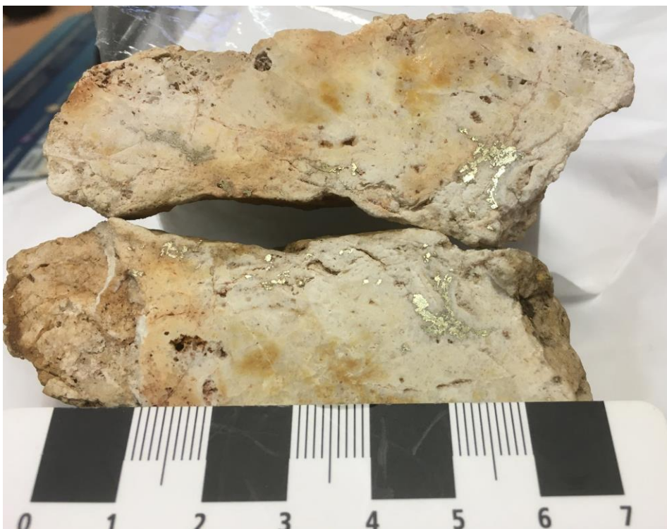
Photo 4: Float sample sawn in half to reveal quartz and pyrite textures
