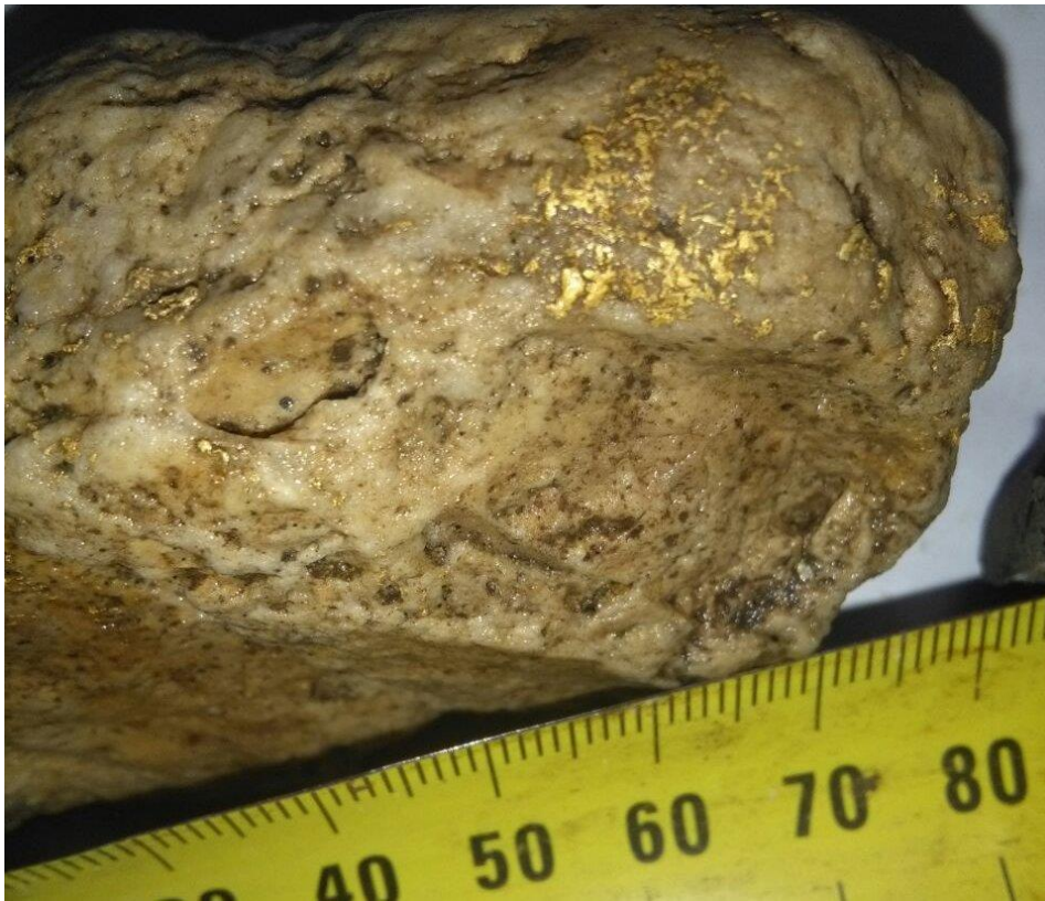
Photo 3: Free gold on surface of quartz-pyrite vein float sample near Pit 200
