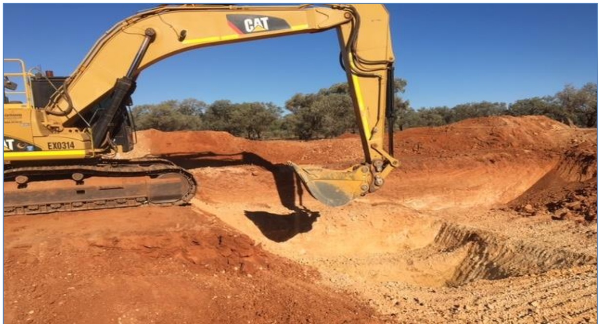
Excavation of 2016 Sample 2 at the site of drill hole ARC647. The pale, beige material is shallow phosphate.
