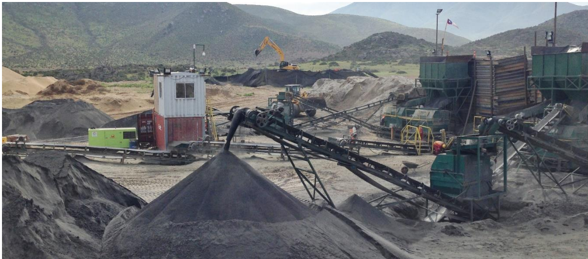
Figure 27. Part of Yerbos Buenas magnetite concentration plant, October 2015. 62% Fe product in closest stockpile and ready for shipping in centre with yellow excavator.
