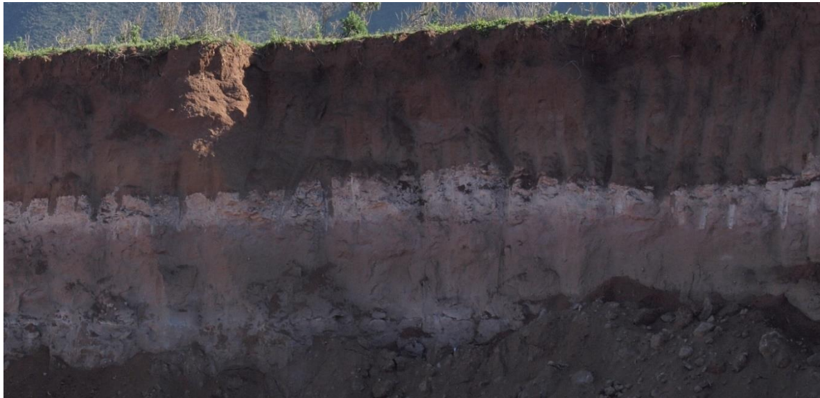
Figure 4 profile of Yerbass Buenas pit wall showing Ferruginous layer, Calcrete layer and underlying Banded Sands layer.
