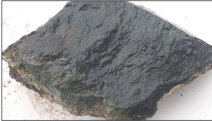
Figure 10: Detail of porphyritic andesite replaced by biotite and magnetite
