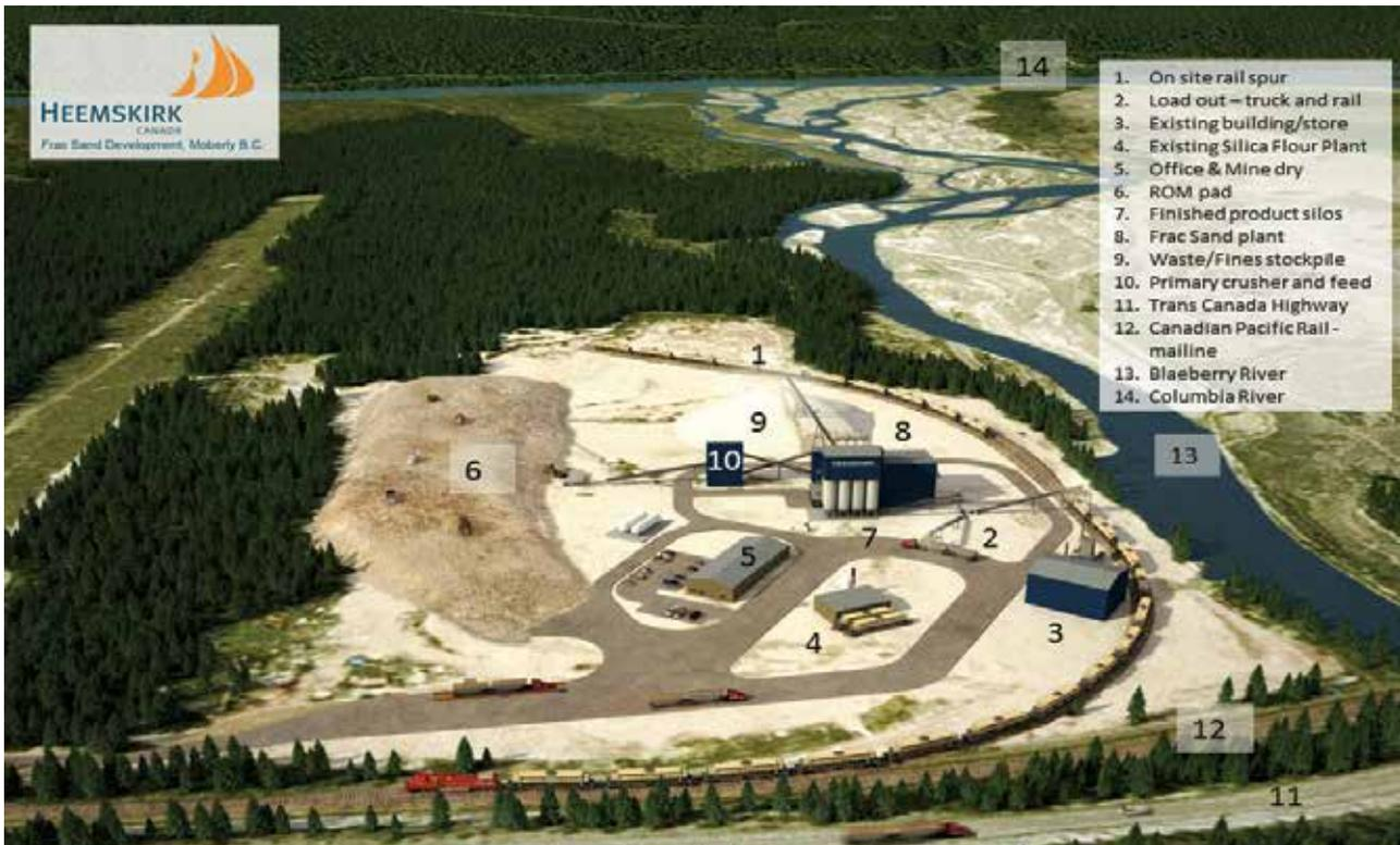
FIGURE 2: LAYOUT OF PROPOSED PLANT AT EXISTING MOBERLY PLANT SITE
