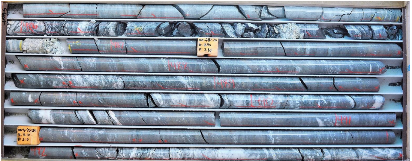
Figure 3 LTED05W1 492.75m to 500.54m down-hole (massive sulphide mineralisation from 492.75m to 493.0m down-hole and semi massive sulphide mineralisation from 494.2m to 495.1m and 496.7m to 500.54m down-hole)
