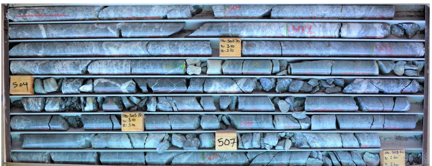
Figure 4 LTED05W1 500.54m to 508.4m down-hole (semi massive sulphide mineralisation from 500.54m to 503.7m down-hole)
