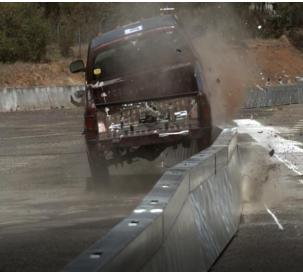
The test was the 100kph test for a 2,270 kg vehicle, impacting at a 25 degree angle. The deflection result was less than 1 metre, which is extremely low for a free-standing temporary barrier, particularly given the weight of this new barrier is half the weight of conventional concrete temporary barriers most commonly used. Our barrier is an unanchored steel and concrete barrier using our patented technology.
