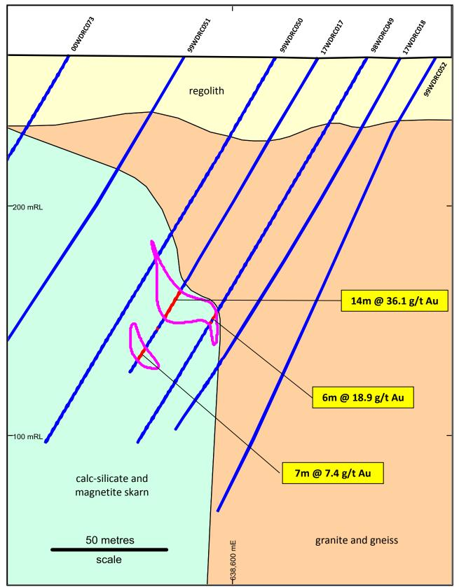
Figure 3. Target 3: 6373170mN Cross-Section with gold drilling results
