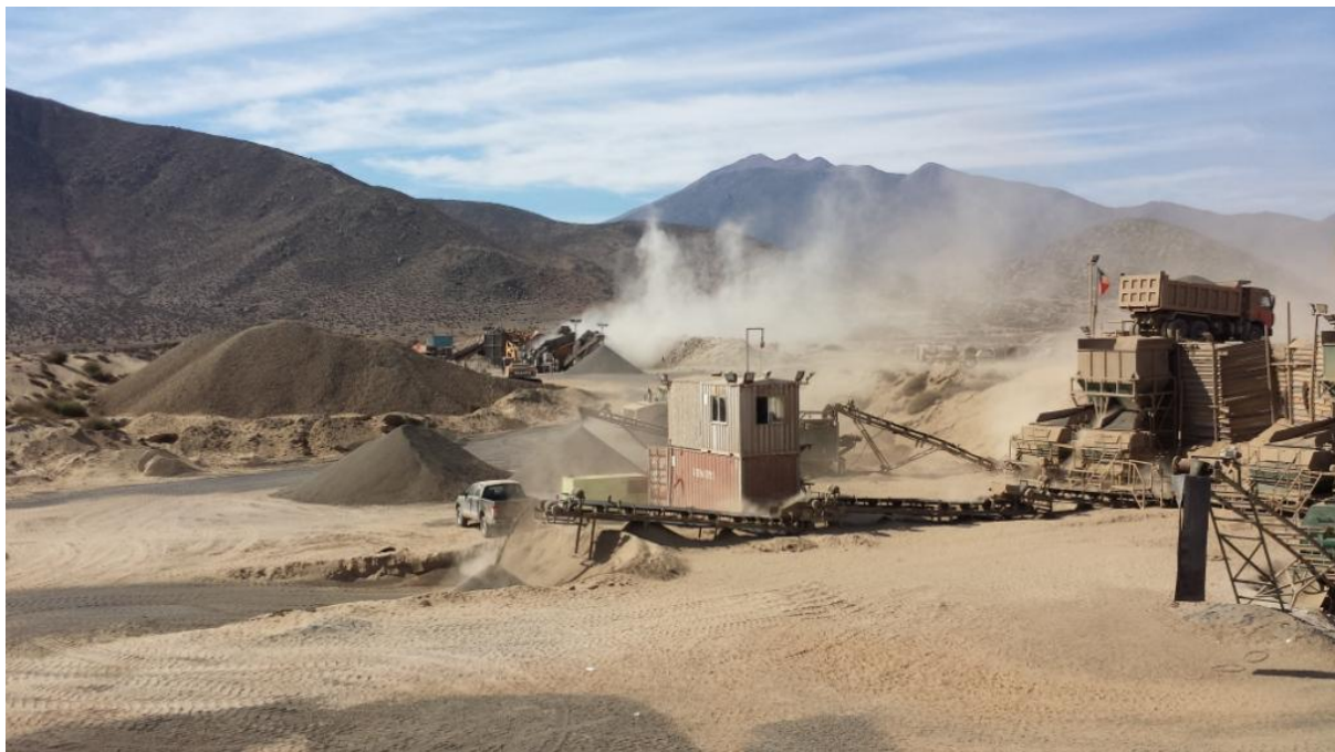
Processing Area with Magnetic Separation Plant in foreground and Crushing Plant in background
