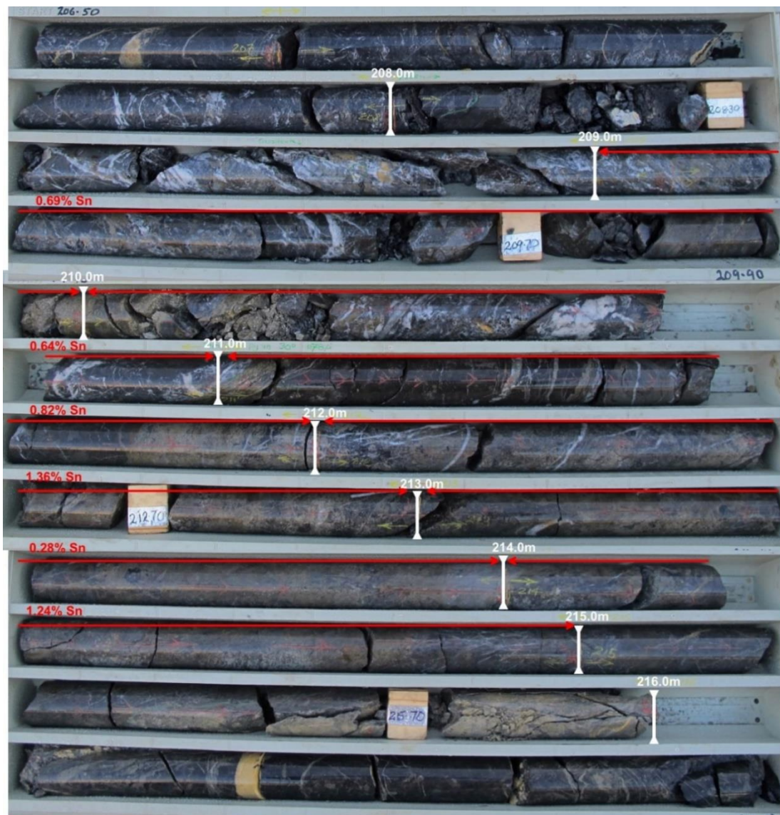
Figure 1: ZQ133 HQ Drill Core Showing 6m Sn Intersection from 209.0m to 215.0m
