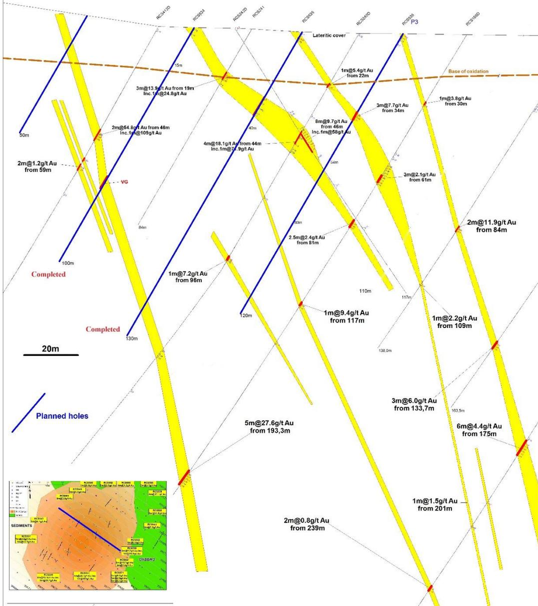
**Figure 2** Makabingui Project Pit 1 - X-Section 99,900N working section with planned holes (blue colour - two already completed)
