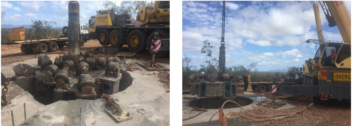
Figure 8 Raise borer head being removed from RAR at completion of ventilation rise
