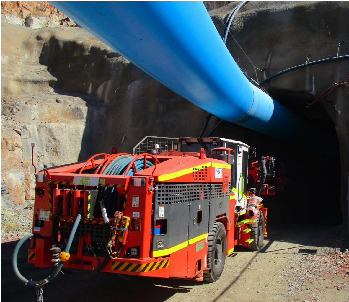
Figure 7 Sandvik Solo DL431 production drill rig heading UG
