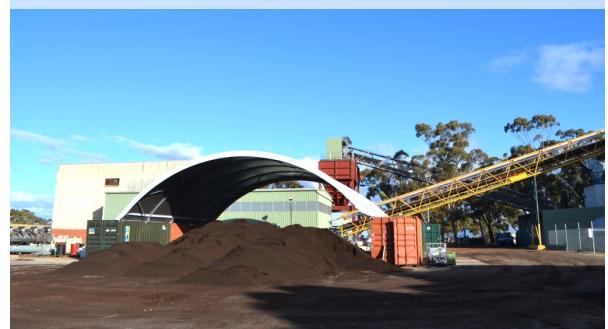
Figure 2 New 'All-shelter' covering the in-ground raw coal bunker
