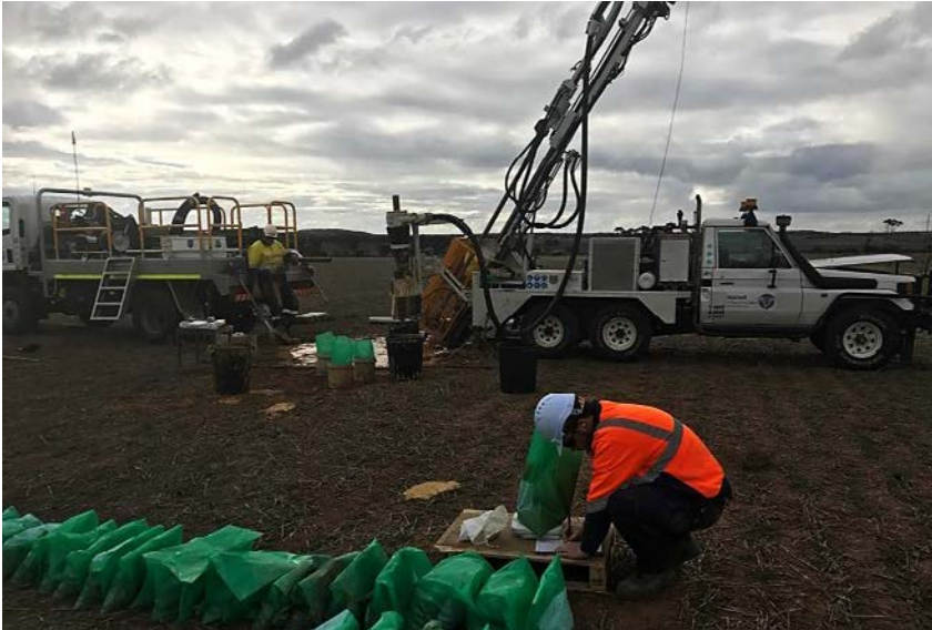
Figure 1 – Aircore rig drilling at Garard's Prospect, Quicksilver Project.
