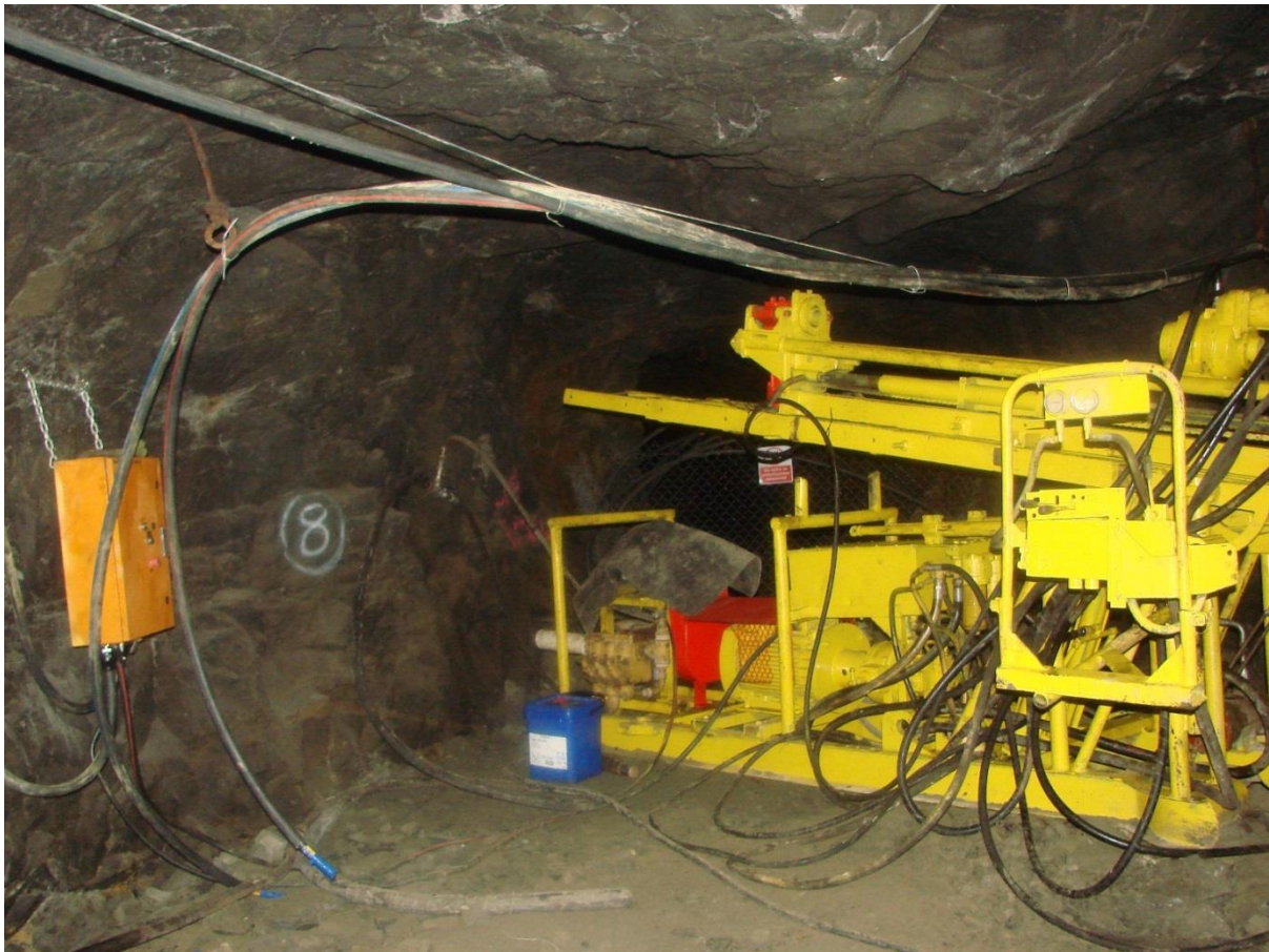
Figure 1: Photograph showing underground drill rig setting up ready to drill.
