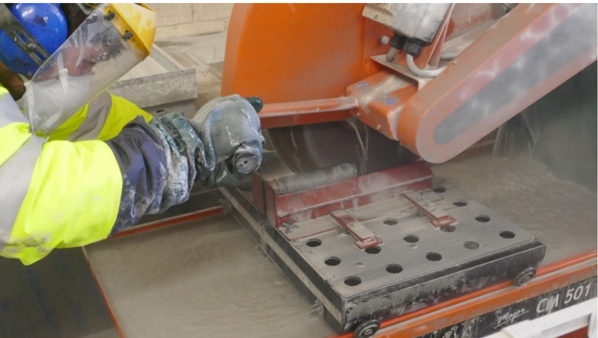
Redmoor drill core being cut prior to dispatch to the laboratory in May
