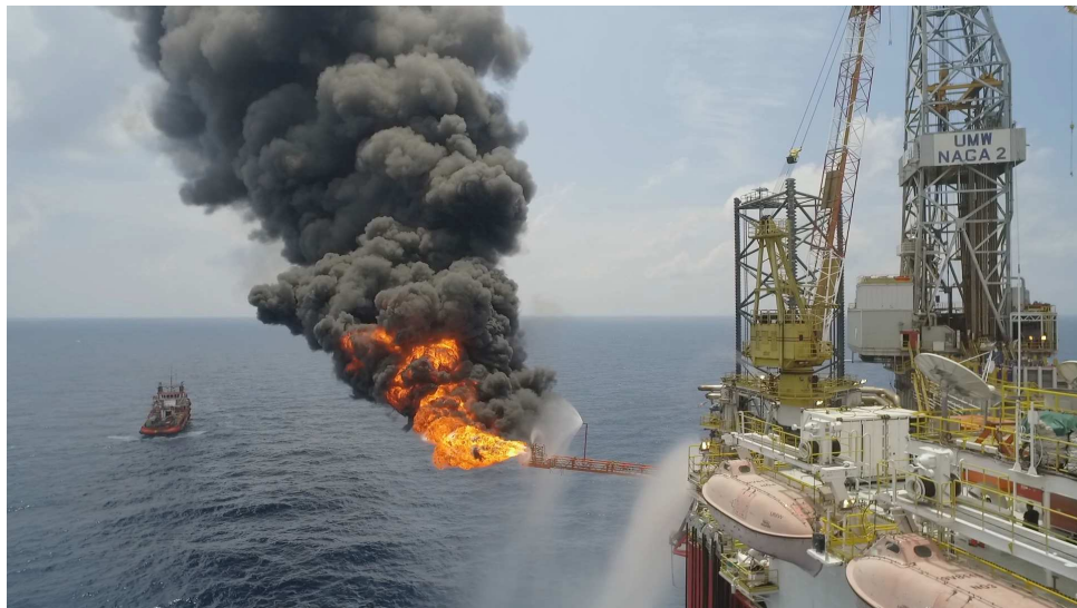
Flow-back to Naga-2 flare boom
