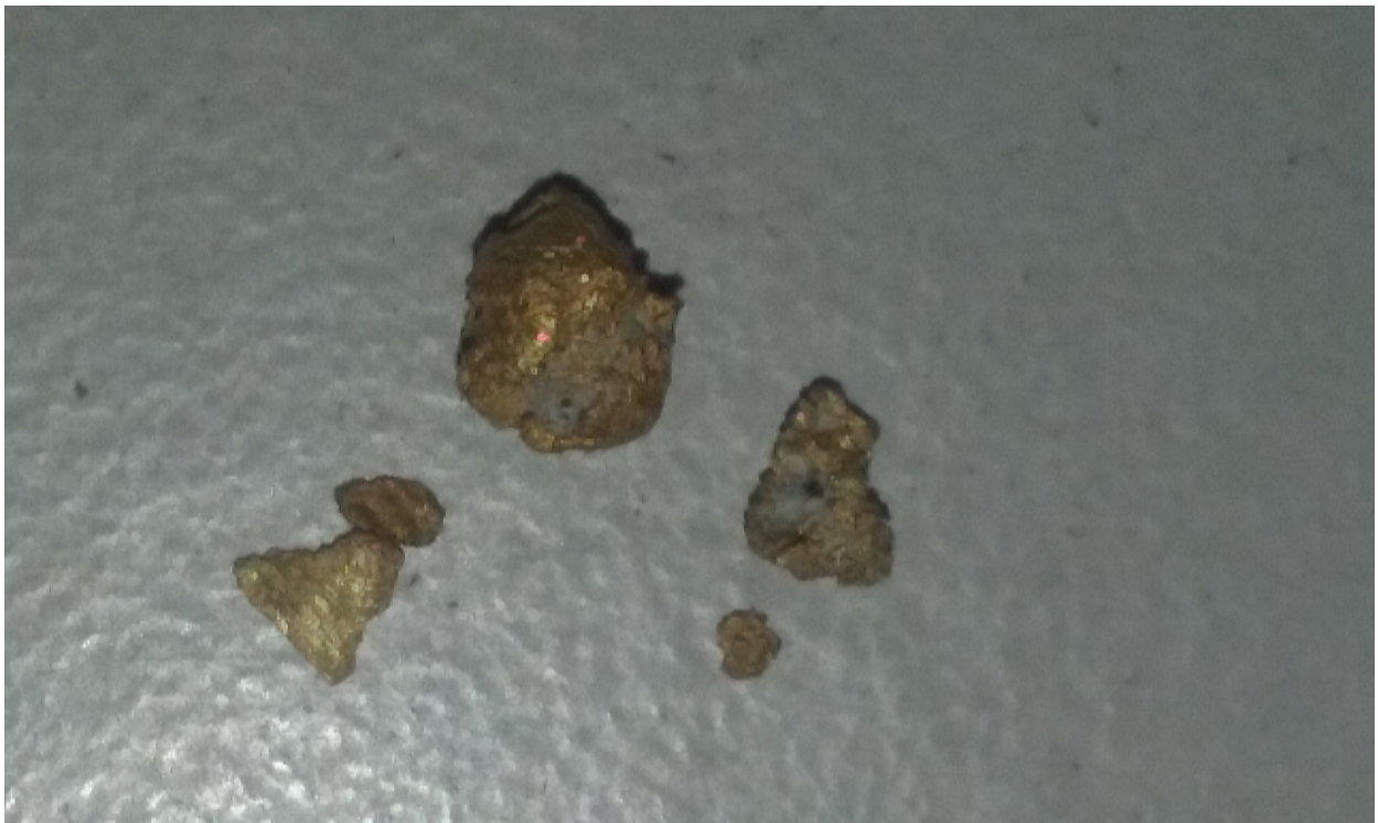
Plate 2: Visible gold in quartz in FERC185 (131-132 metres). Grains are approximately 2 to 3mm in size. One metre sample assayed 313g/t Au.
