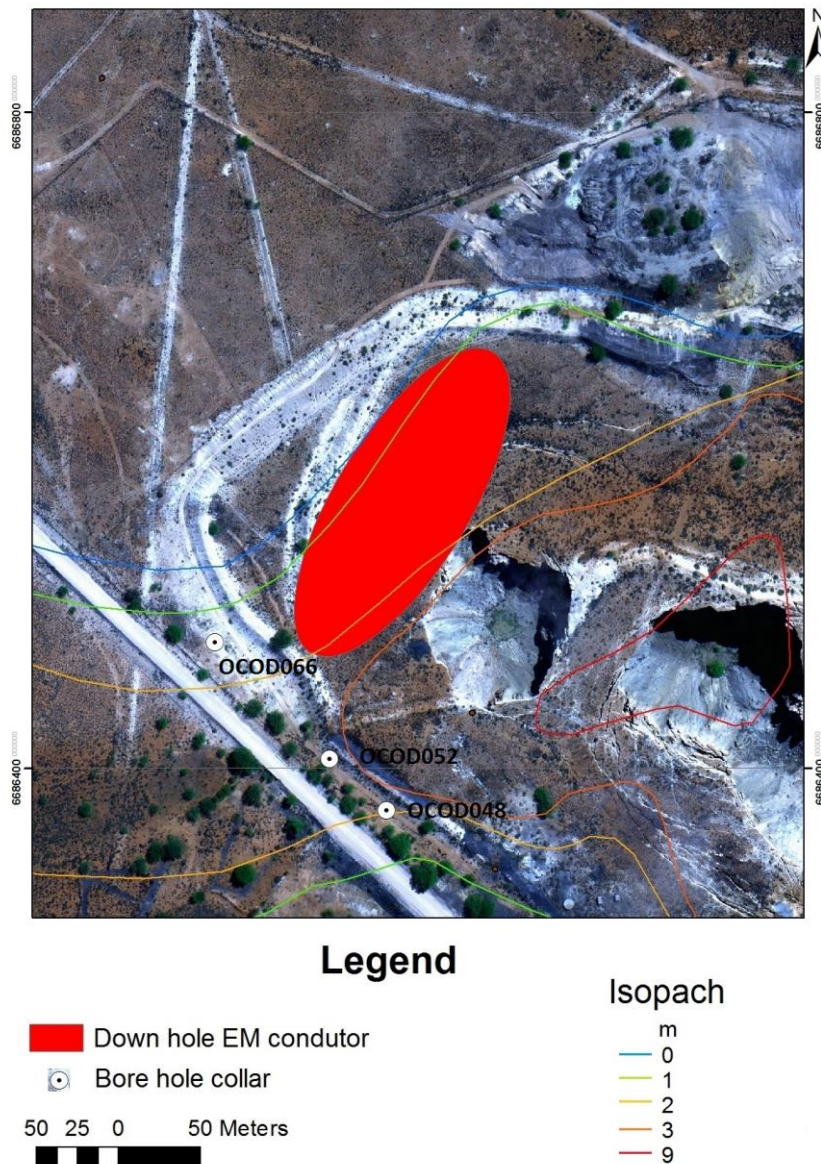
Figure 7: Plan showing position of the down hole EM conductor detected in OCOD066.
