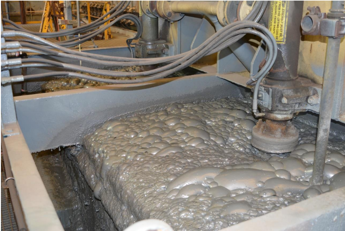
Figure 2 Zinc flotation cells
