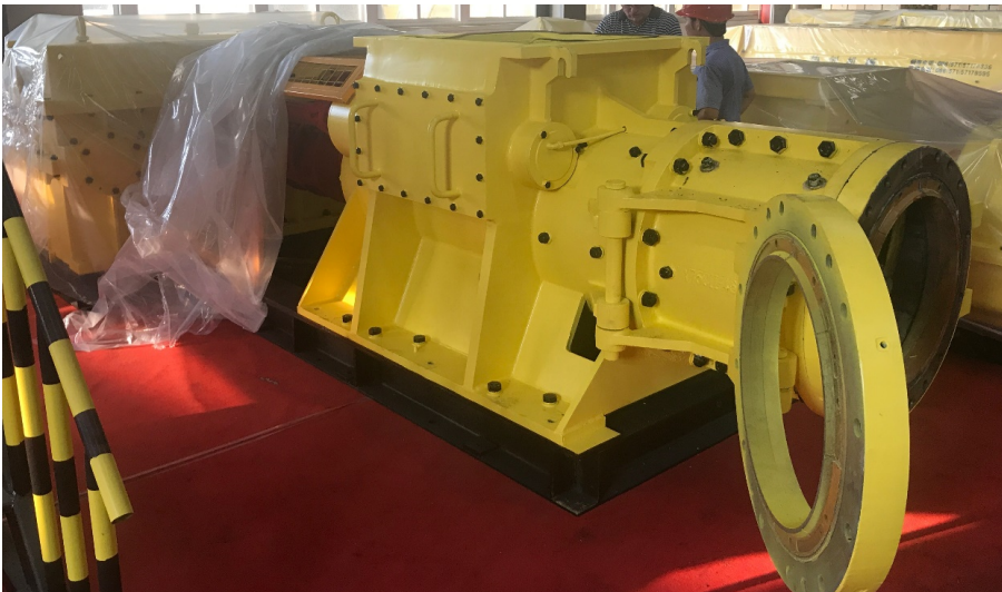
Photo above: New larger scale extruder which will be assembled inside the Primary Processing building at the Bacchus Marsh HVFT, creating a second line of production alongside the existing machine.
