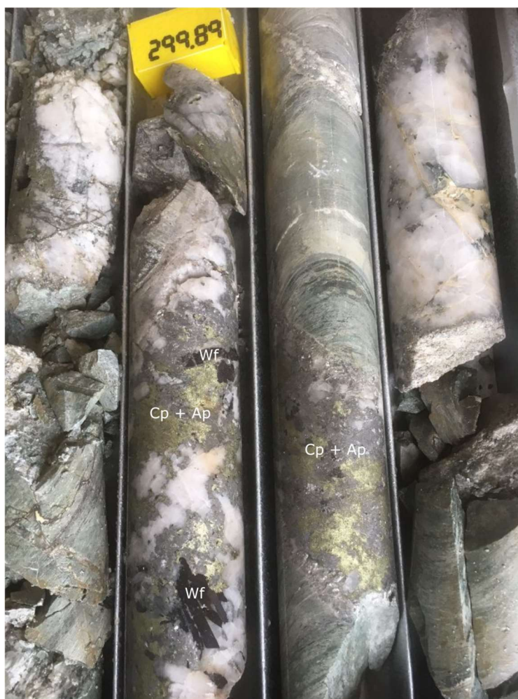
High grade vein mineralization within SVS (CRD009 from 229.00 m – 302.00 m, only part of section visible. Wf = wolframite, Cp = chalcopyrite, Ap = arsenopyrite
