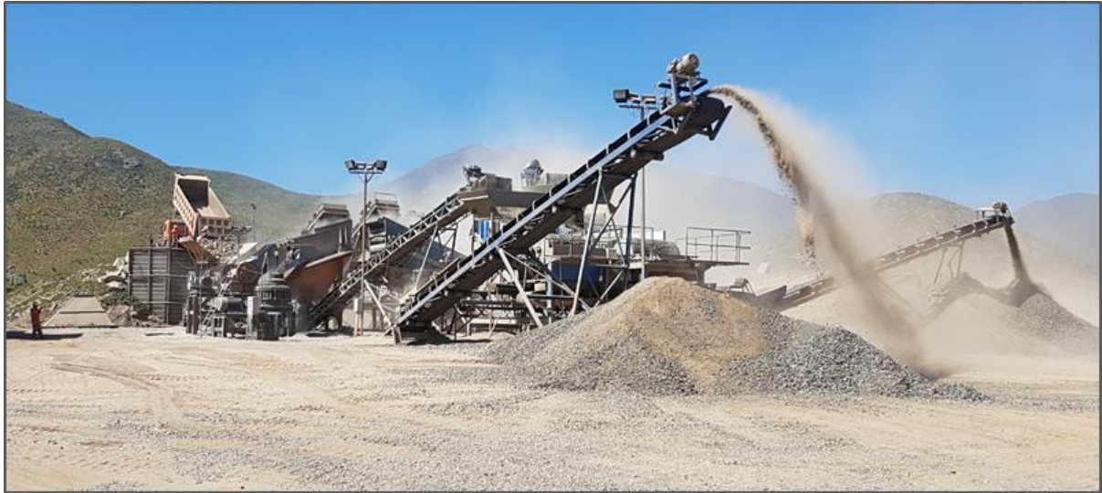
Figure 2 – Crushing plant Line N° 1 and 2 showing -32mm pre-concentrate stockpiles
