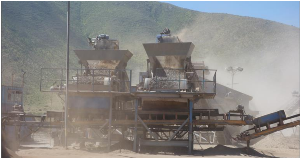
Figure 1 - Reconfiguration of Line N° 1 and upgrading of Line N° 2 completed – image shows Belt-Drum magnets that produce the pre-concentrate feed to the magnet plant.
