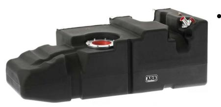
Frontier long range plastic polymer fuel tanks have been very well received by the market due to their durability and light weight. Once again, the range has been expanded to suit many vehicles.
