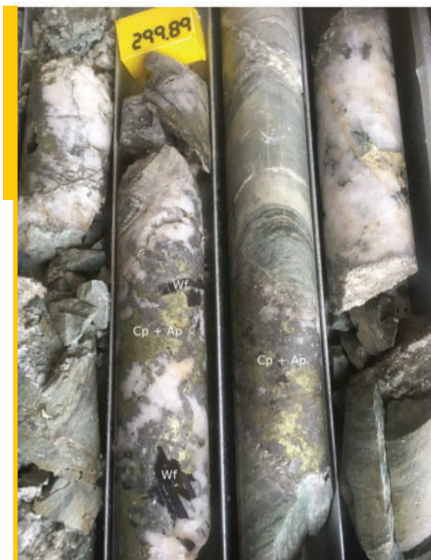
High grade vein mineralization within SVS (CRD009 from 229.00 m – 302.00 m, only part of section visible. Wf = wolframite, Cp = chalcopyrite, Ap = arsenopyrite
