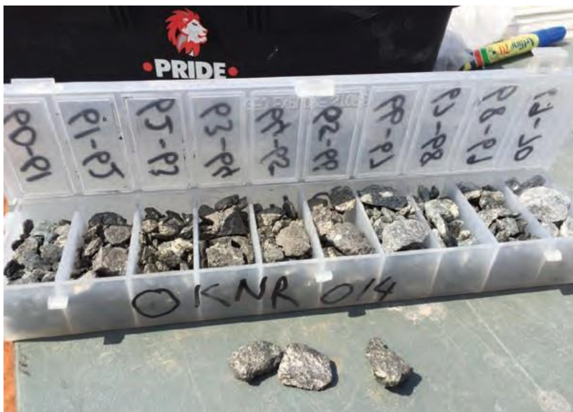
Figure 15: Massive sulphides in OKNR014 which returned 7m at 6.45% Zn and 0.43% Cu from 60m.
