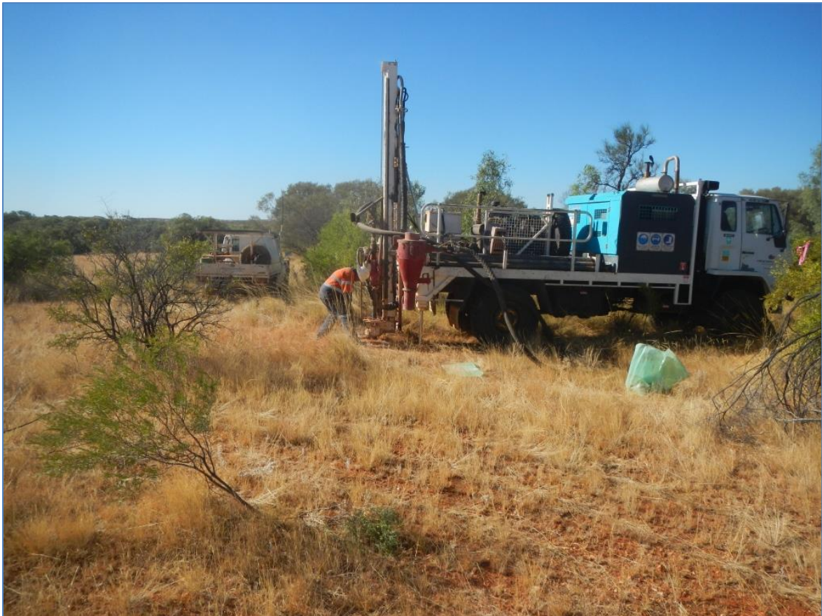
Figure 4. Low environmental impact drilling in progress at Rockhole. No tracks or drillsites were cleared.
