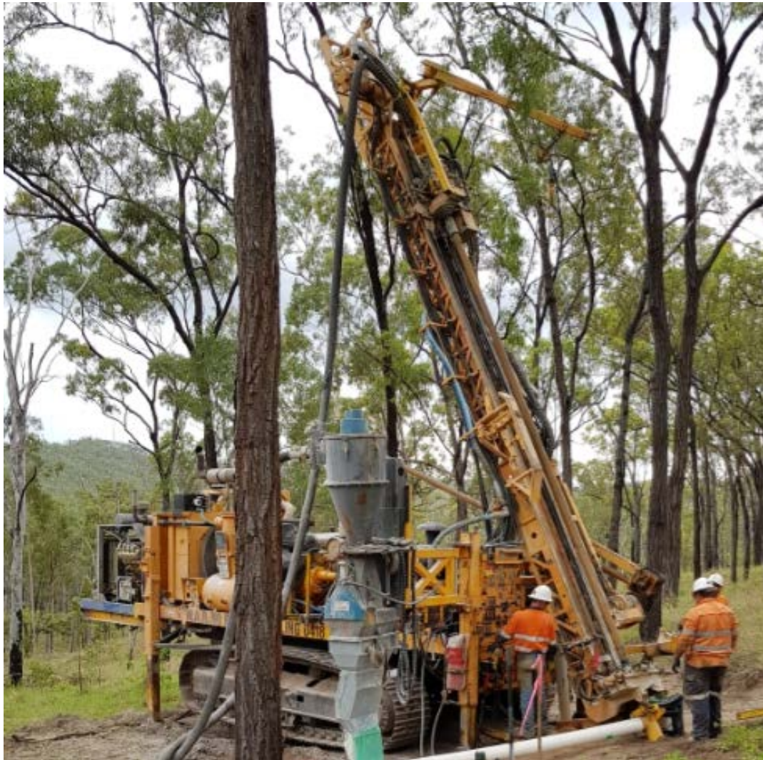
RC drilling rig at New Constitution prospect, Triumph project, SE Qld.
