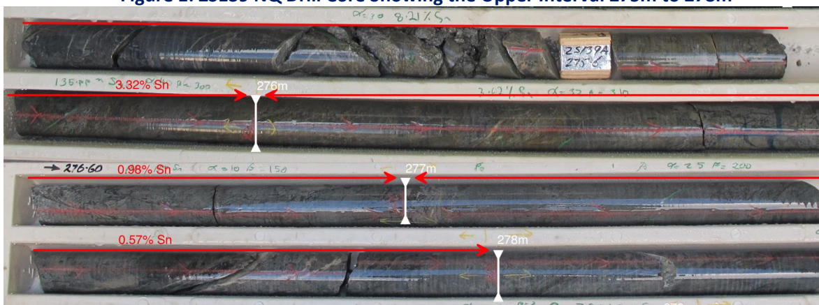
Figure 1: ZS139 NQ Drill Core Showing the Upper Interval 275m to 278m
