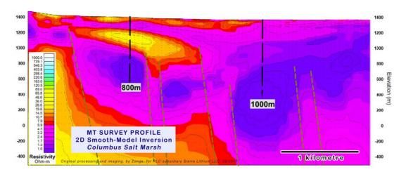
The potential lithium brine targets selected for drilling on the Big Smoky South project are shown in the MT survey profile below. The deeper of the two drill holes is a 1,000 metre deep hole designed to test a substantial target extending from 600 metres below surface identified in the Company's MT survey data.
