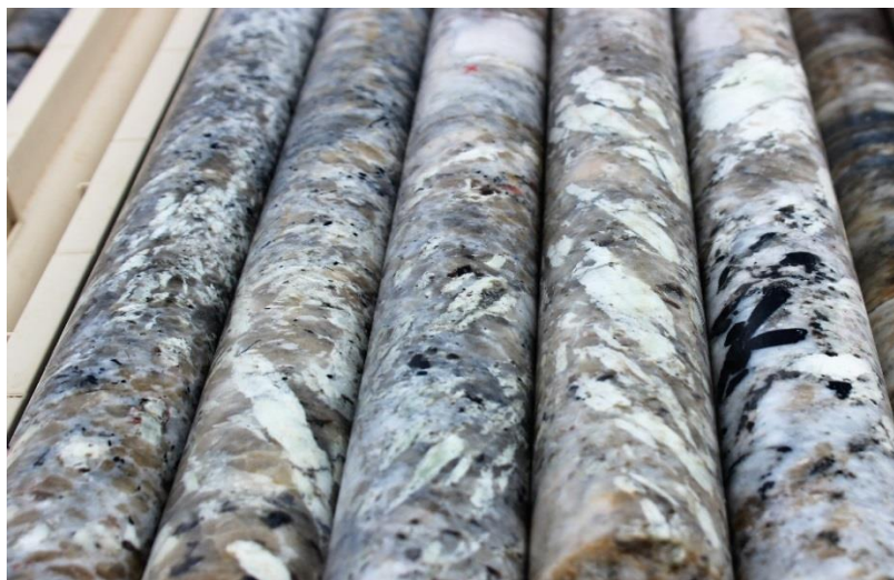
Image 3: Core from KEGM051 with coarse grained spodumene throughout a wide interval.
