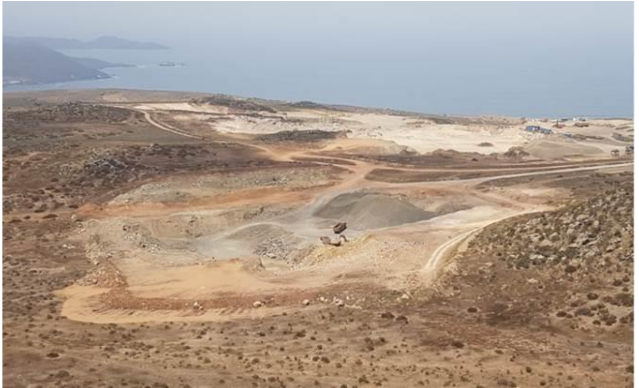
Figure 2 – General view of complete trial mining pit showing deepening pit and commencement of third bench
