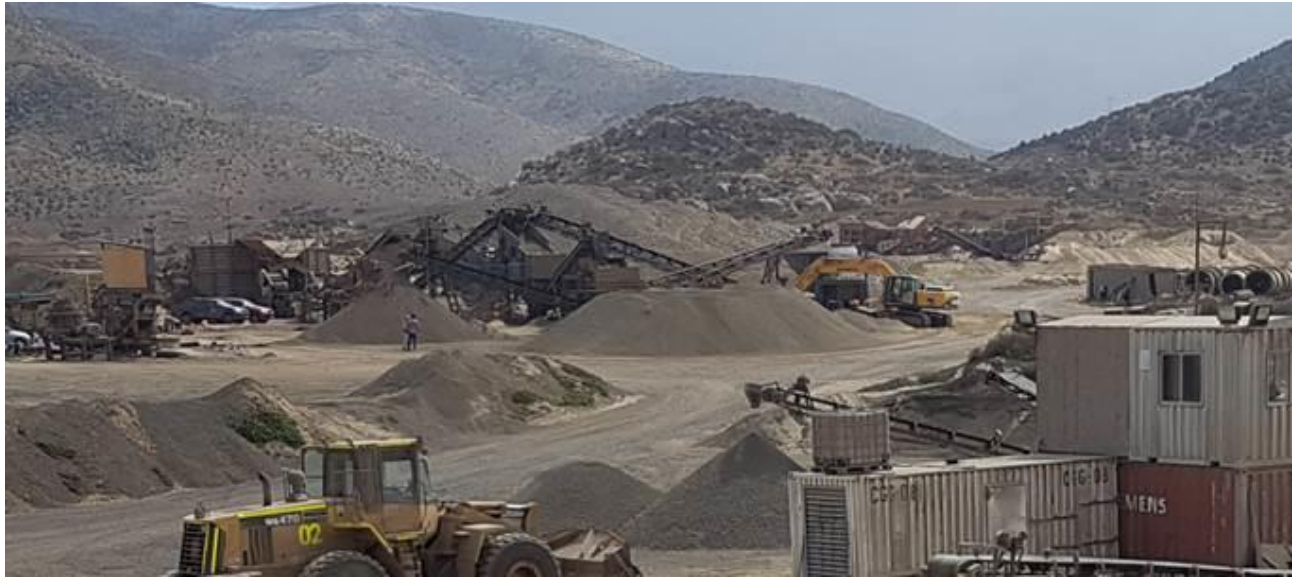
Figure 4 – Demonstration crushing plant showing pre-concentrate stockpiles ready for treatment in magnet plant
