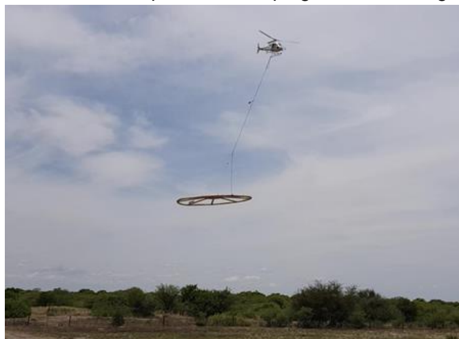
Figure 1 - Airborne Magnetic and EM Survey undertaken over GWD1 Prospect
