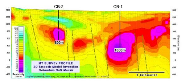
The 2 drill holes for which permits have been issued at Columbus Salt Marsh project are shown on the MT (magneto-telluric) survey as CB-1 and CB-2. In this profile resistivities of less than 1 ohm-m are represented in the colours red, purple and blue (refer to scale on LHS). The planned drill hole (CB-1) is shown targeting the upper 400 metres of the large zone of resistivity less than 1 ohm-m between 600 metres and 1,600 metres depth (shown coloured blue, purple and red in the section).
