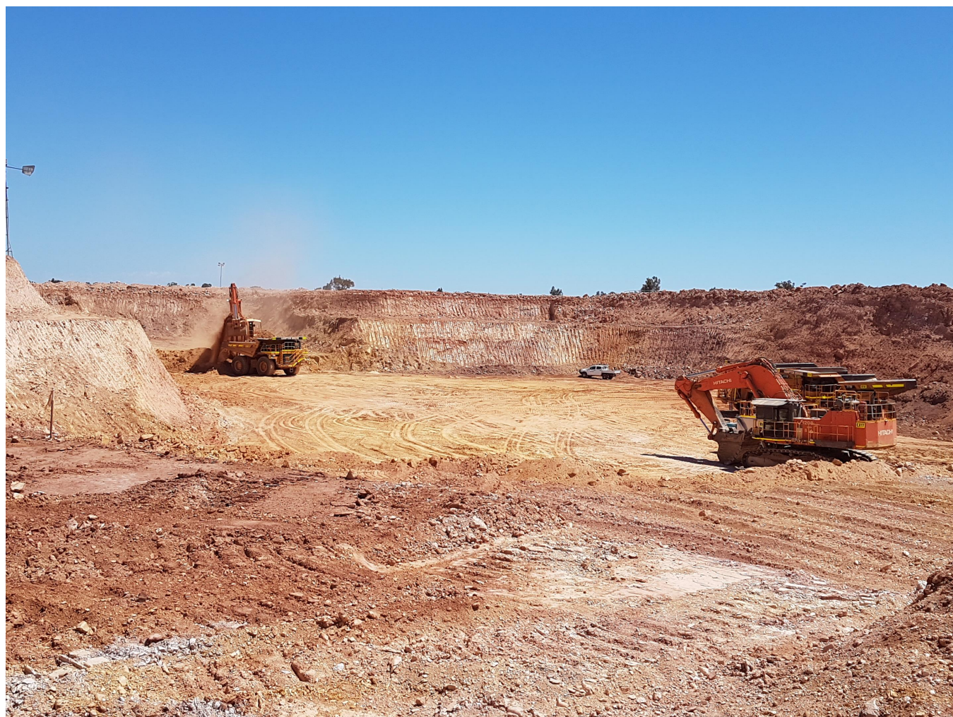
Figure 2. Mining at the Trouser Legs Gold Mine – 2 x 120 Tonne Excavators, 4 x Cat 777 Dump Trucks in Pit
