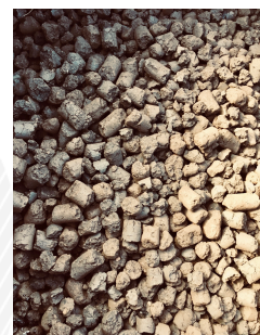
Pictures (above, left to right): 20-foot shipping container loaded with Coldry solid fuel, destined for testing in Tasmania. View through the top loading point & close up of Coldry pellets.
