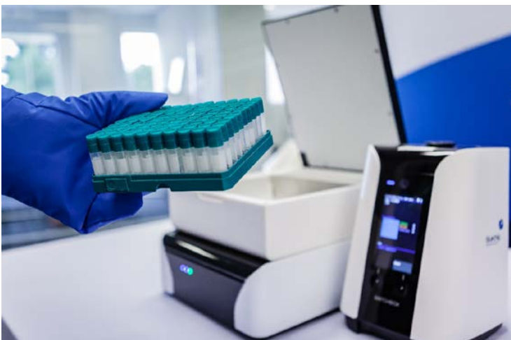
Bluechiip Matchbox, Multivial Reader, Cold Top and box of 100 vials
