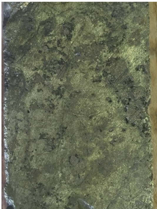
Figure 2 – Core photographs of exceptionally high grade ‘including’ intercepts: L - CRD018, 358.72m, solid chalcopyrite with wolframite (interval contains 10.73% Cu and 3.42% WO 3 ); R - CRD019, 510.95m, solid wolframite (interval contains 8.58% WO 3 )
