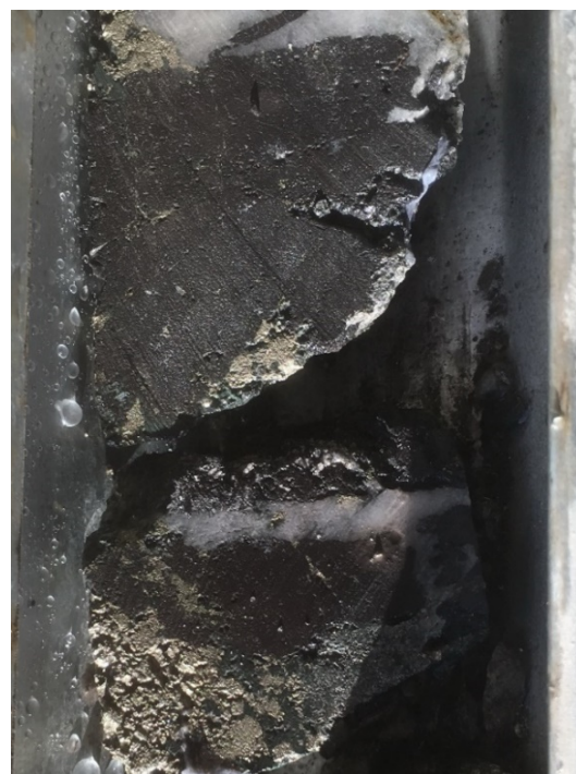
Figure 2 – Core photographs of exceptionally high grade ‘including’ intercepts: L - CRD018, 358.72m, solid chalcopyrite with wolframite (interval contains 10.73% Cu and 3.42% WO 3 ); R - CRD019, 510.95m, solid wolframite (interval contains 8.58% WO 3 )
