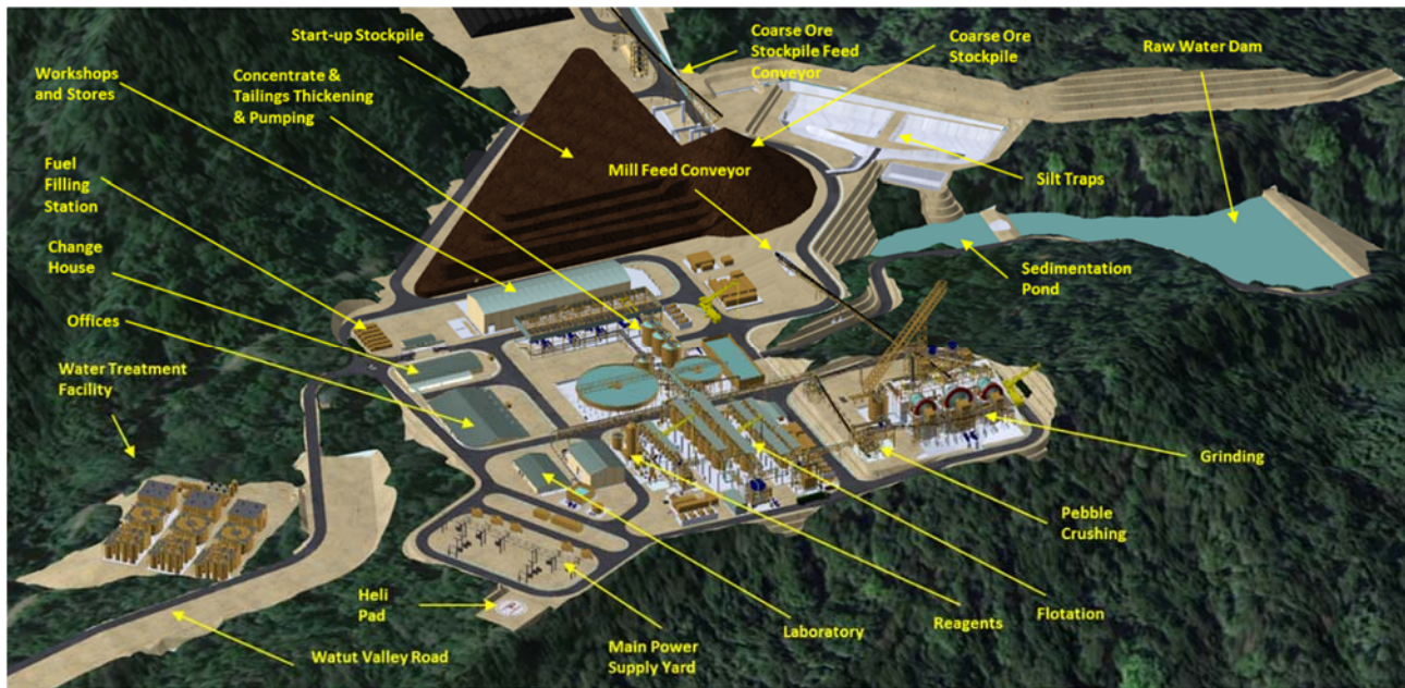
Figure 4: Proposed Watut Process Plant
