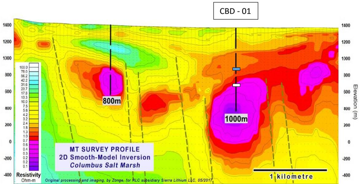
Drilling underway – downhole depth as at Friday 23 March is shown by the white box on CB-1. The blue box shows the approximate interval pump tested and sampled. Note that resistivity is the inverse of conductivity i.e. low resistivity equals high conductivity.
