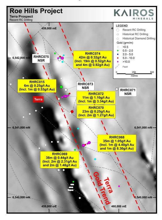
Figure 3: Terra Prospect, recent gold focused RC Drilling
