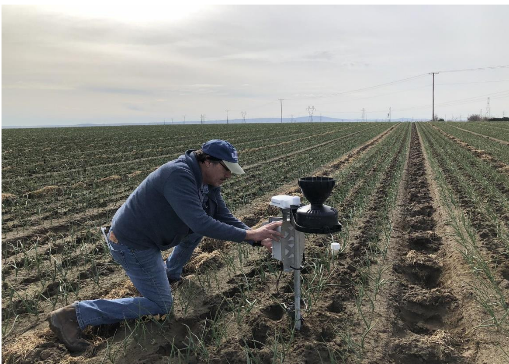
Figure 2: CropLogic agronomist installing probe in an onion field in Washington State, USA
