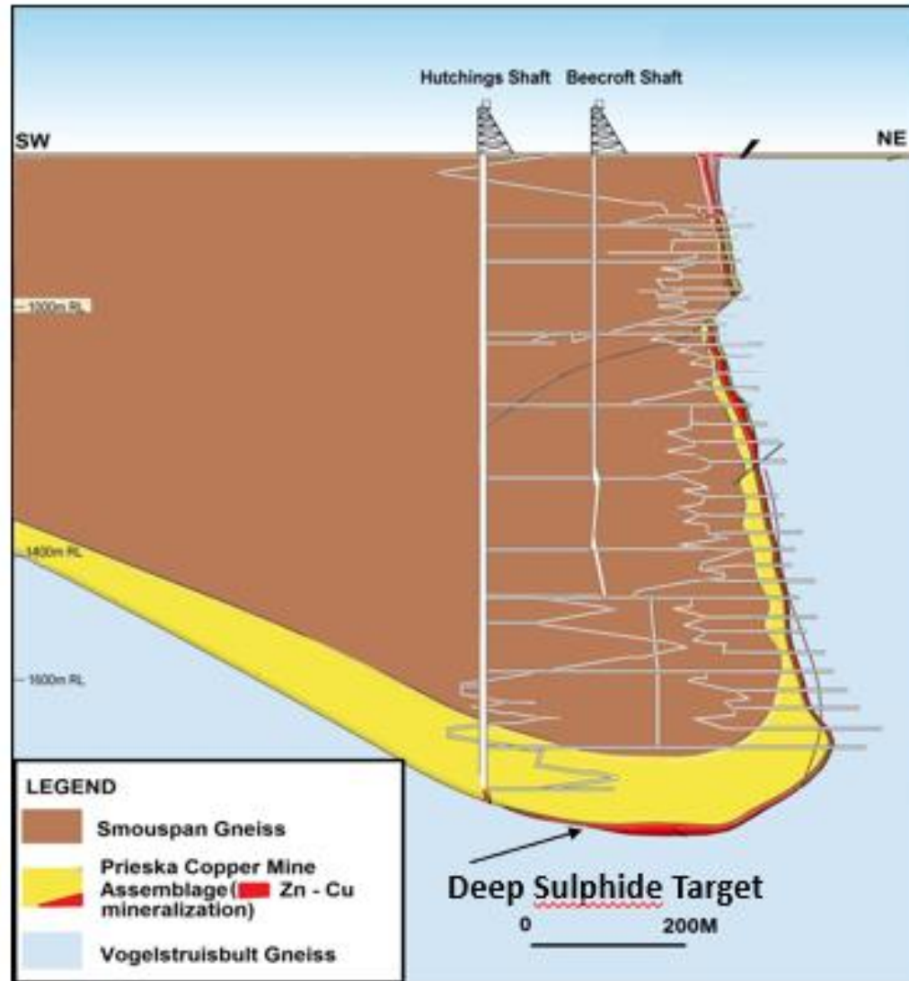
Appendix 2 Figure 2: Simplified geological section through historic Prieska Copper Mine showing structure and locality of the Deep Sulphide Target below the old workings. The Vardocube Massive Sulphide Target is the southeastern strike extension of the Deep Sulphide mineralisation (refer ASX release 8 February 2018).
