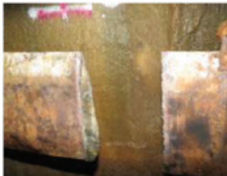
Location of removed section from underground bunton
