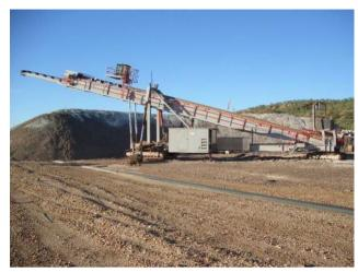
Figure 7 - Stacker infeed conveyor
