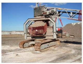
Figure 8 - Crawler-mounted radial stacker conveyor
