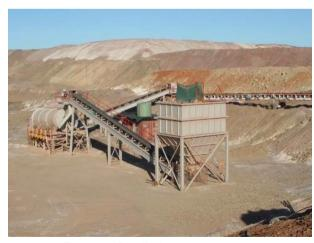
Figure 3 - Bin discharge conveyor
