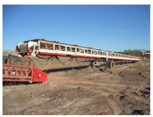
Figure 5 – Agglomerator discharge conveyor
