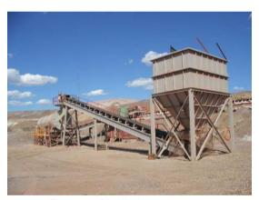
Figure 2 - Bin discharge conveyor
