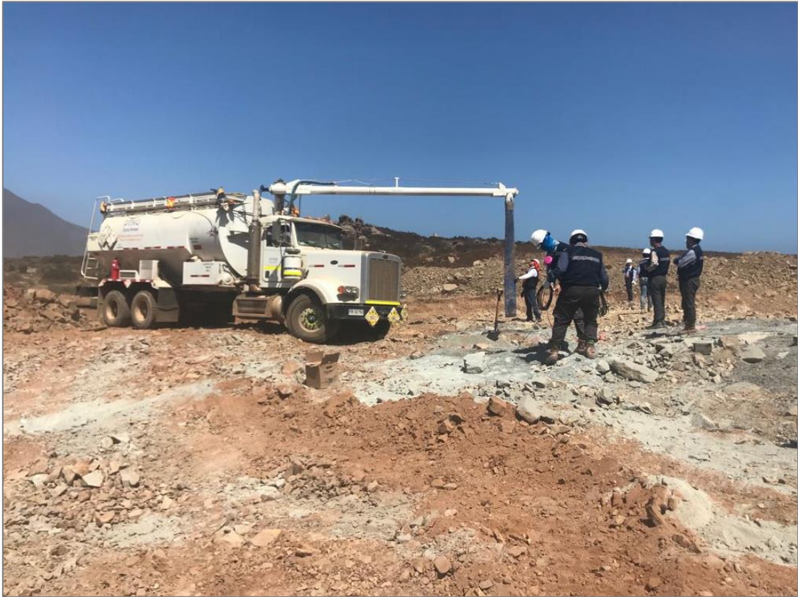
Figure 3 - Hanwha loading emulsion explosives ready for blasting
