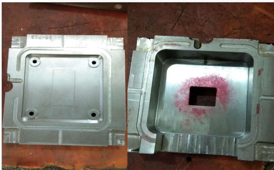
Fig 1. Xped SH2 Gateway Injection Mould Tooling
