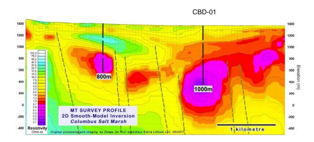
The presence of brine was successfully confirmed by a pump test conducted approximately 200ft (61m) above the Target Zone in CBD-01. An aquifer within a zone of tuff and volcanic ash deposits from 1642ft (500m) to 1742ft (531m) was pump tested and sampled. Assays detected no lithium in the brine sampled at this level (ASX release 26 March 2018).
